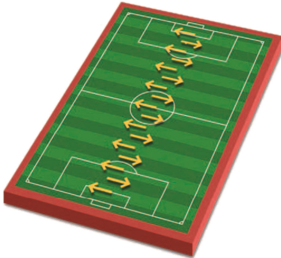
Direction the rolls have been installed in.
