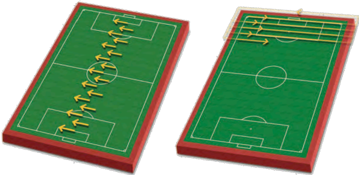
Direction the rolls have been installed.
