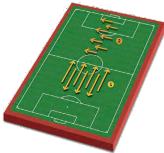
Direction of travel for maintenance of ageing turf. The final pass must always be against the installation direction.
