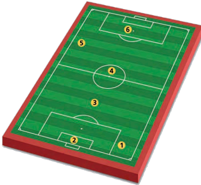
FIFA measuring points for ball roll test
