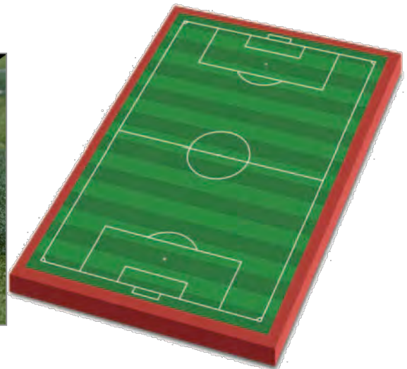
Rolls of turf installed in opposite directions
