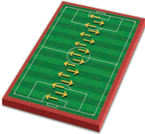
Direction the rolls have been installed in.
