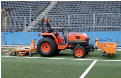
Unit with fixed brush and needle bars
