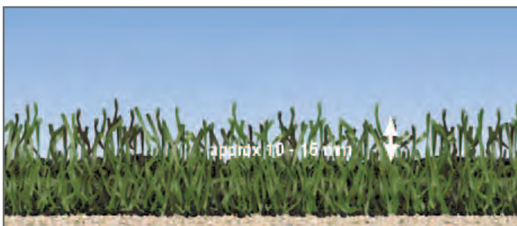
Pile projection length for texturised fibres
