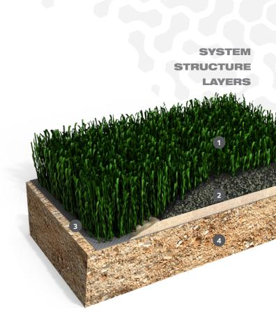
60mm pile height exclusive Polytex mono-filament sports yarn – incorporating spring-back technology for highest durability and play characteristics.
