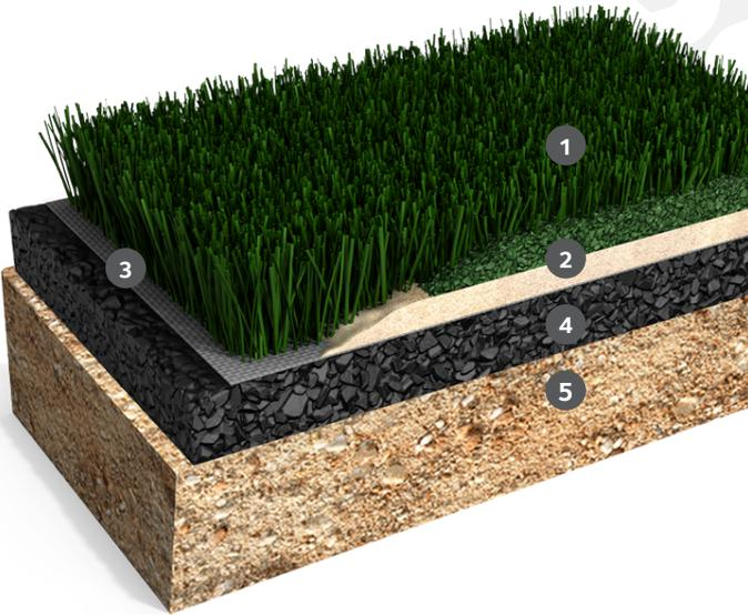
**1** 40mm pile height exclusive Polytex mono-filament sports yarn – incorporating spring-back technology for highest durability and play characteristics.
